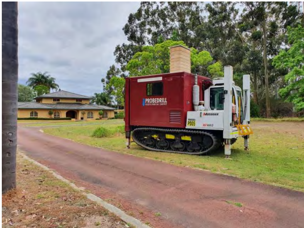
Photograph 4: CPT testing near the centre of the site
