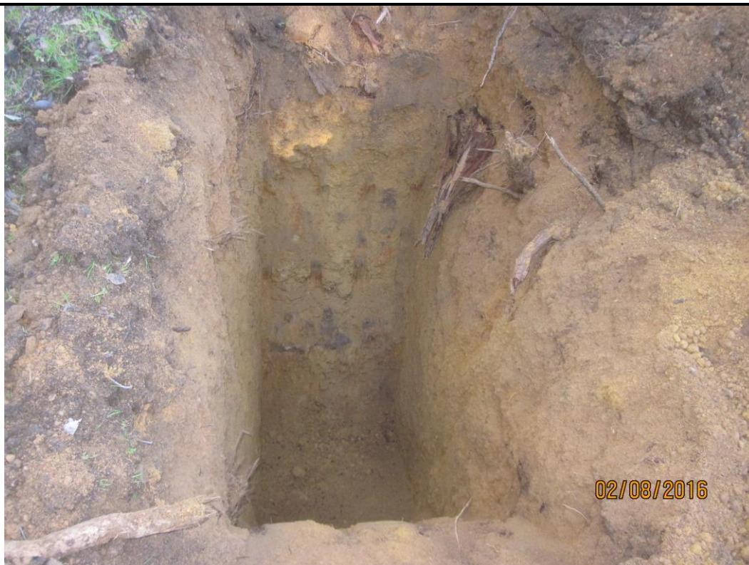
Photo 5. Soil Profile of Test Pit location 01 (TP1)
