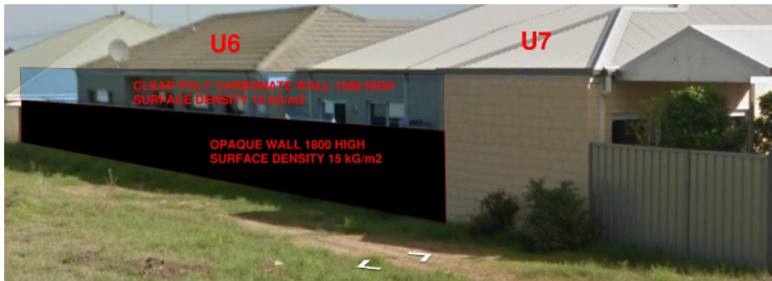
FIGURES L.1 – LOADING DOCK NOISE WALLS
