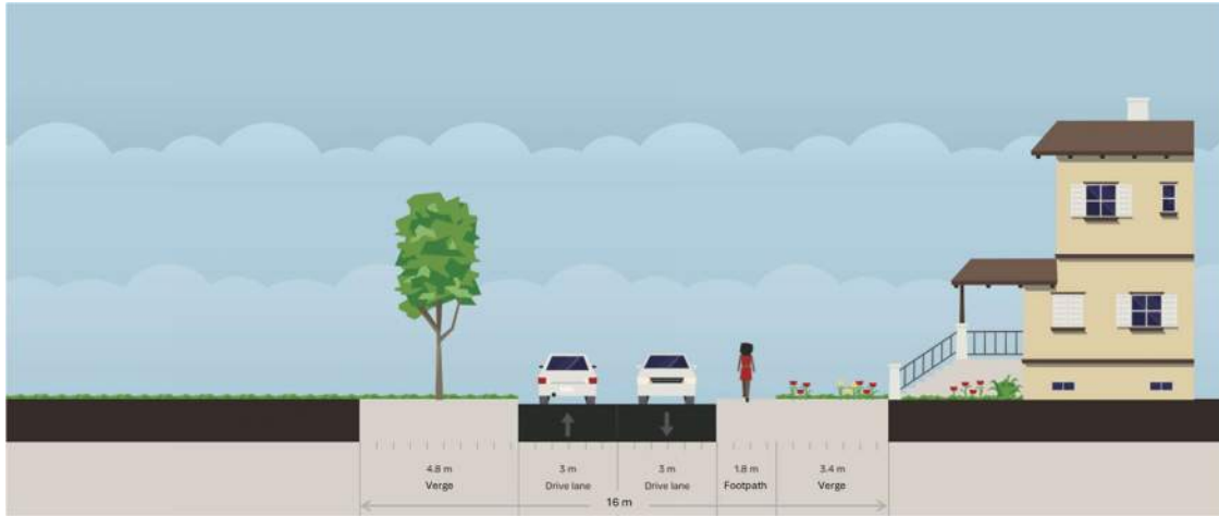
Figure 14 Indicative Cross Section – Proposed Road adjacent to Public Open Space and Residential (16m Reserve)
