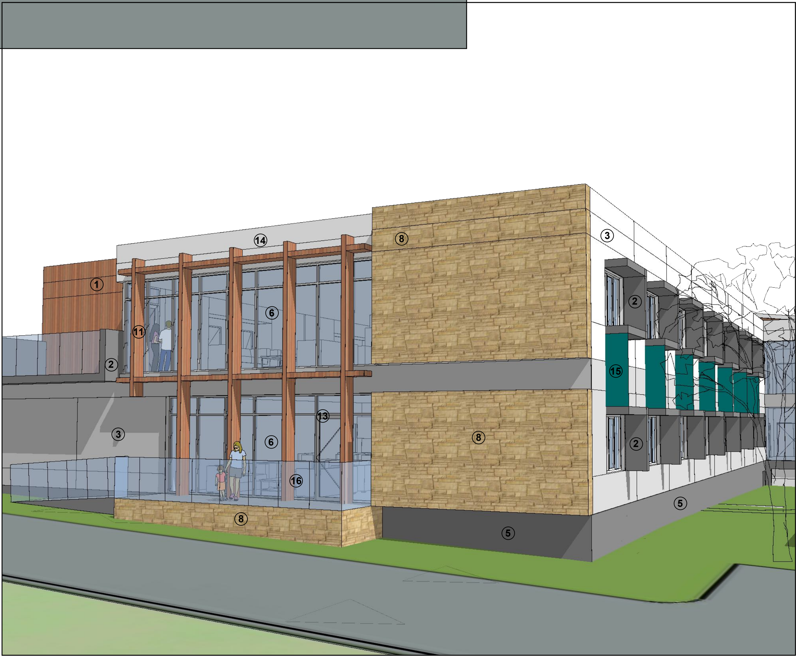
VIEW TO BUILDING REAR ENTRANCE - WITH MATERIALS INDICATED
